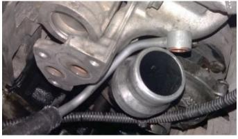
In this point of the assembly, is where **the importance of the flexible area of the pipe resides,** since if it's totally rigid it wouldn't be possible its installation.
