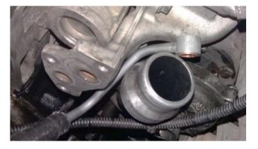
6) Place the pipe in the proper position in the turbocharger and screw it slightly without tightening it. In this step make sure that the copper washers are correctly positioned.
