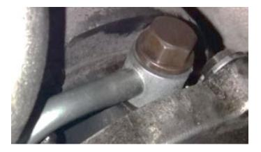
The technologies and materials used by the manufacturers for this flexible zone are diverse. **Ajusa uses a flexible pipe made of elastomer** formed together with the use of a thermal sheath that increases even more the resistance
